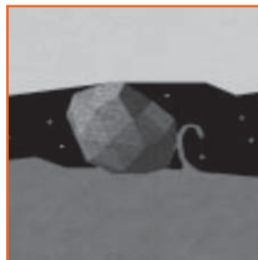
Figure 2: Grinding from contaminant particles can wear channels or grooves into the smooth surfaces of rods and cylinders.
